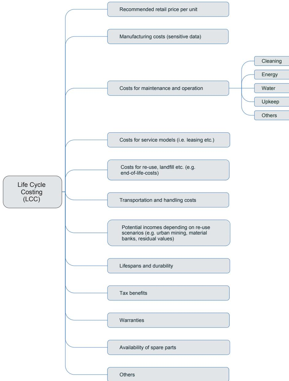
Figure 25: Overview of data requirements for Life Cycle Costing (LCC)
