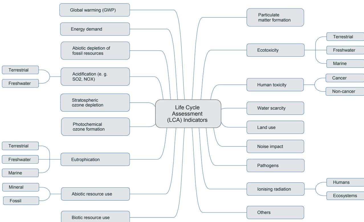
Figure 24: Overview of indicators in an LCA
